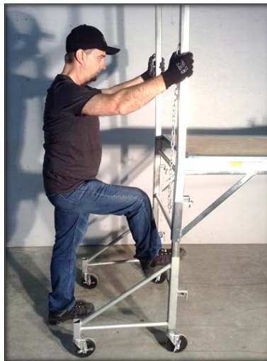
2. Always maintain 3-point contact when climbing CS1 ladder frame. NOTE: Outriggers must be in place prior to climbing.
